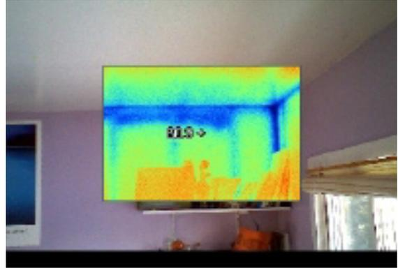
Figure 4: Properly installed cellulose is an excellent insulation. Unfortunately it is often poorly installed with missed areas and settling the most common quality problems.
