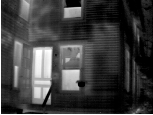
The quality of the images produced by modern IR systems is remarkable. Missing and poorly installed insulation is easily seen.
